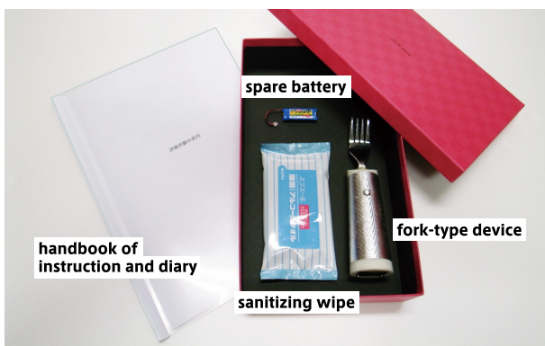
Fig. 7 Fork-type device set complete with instruction manual, diary, spare battery, and sanitizing wipe.
