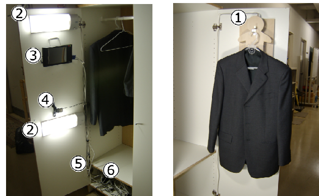
figure 2: Prototype of TagTansu. (1) hook sensors, (2) lights, (3)LCD, (4) USB camera, (5) a magnet switch, (6) a host PC.
