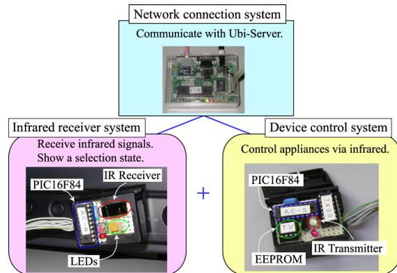
FIG. 5. *System architecture of Attachable Controller.*
