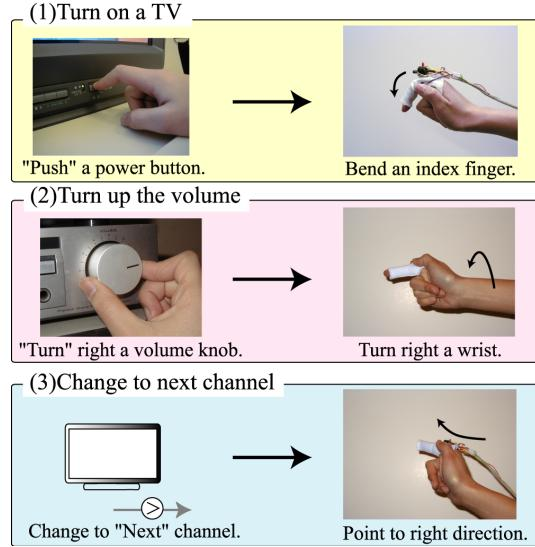
FIG. 6. Examples of operations using Ubi-Finger.
