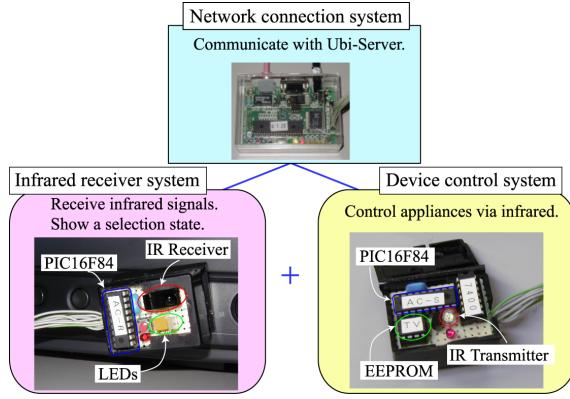
FIG. 5. System architecture of Attachable Controller.
