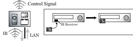
FIG. 4. Basic concept of Attachable Controller.
