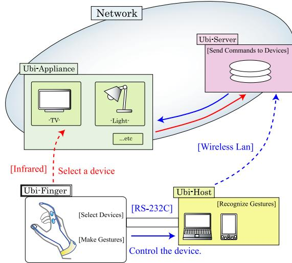
FIG. 2. System architecture of *Ubi-Finger*.
