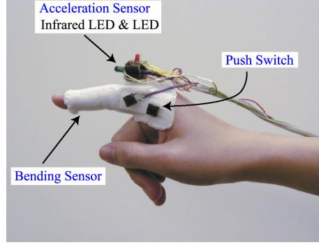
FIG. 3. Prototype of Ubi-Finger hardware.
