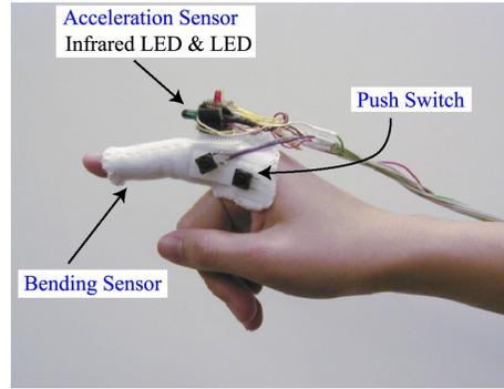
FIG. 3. *Prototype of Ubi-Finger hardware.*
