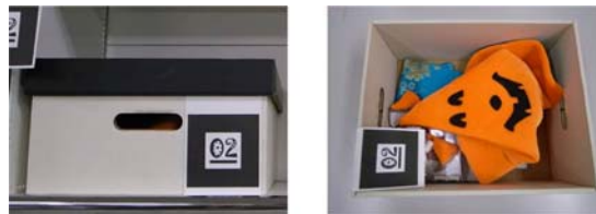
Fig. 2. Example of a storage box with visual markers. ARToolKit visual markers are attached inside/outside boxes.
