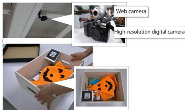
Fig. 4. Capturing photos of boxes by a fixed camera. Users can easily capture an image of the items stored in a box only by putting the box on the photo space.
