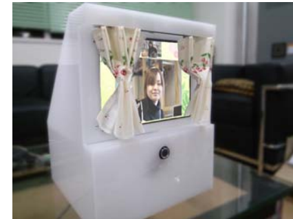
figure 1. SmoothCurtain video communication system. Small curtains hung in front of the monitor control privacy.
