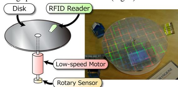
**Figure 2.** The prototype IODisk.
