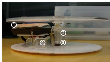
**Figure 3.** Device architecture. (1. RFID reader, 2. low-speed motor, 3. rotary sensor, 4. full color LED)
