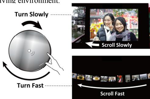
**Figure 1.** The concept of the IODisk. Users can control the speed/direction of digital contents in proportion to the rotating speed/direction of the disk.
