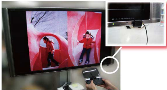
Figure 6. Sensor placement on TV IR port.
