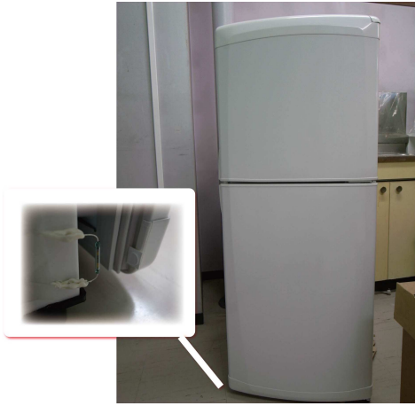
Figure 5. Sensor placement on refrigerator door – Lab B.
