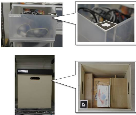
Figure 3. Examples of storage boxes and visual markers. We attached ARToolKit visual markers inside drawer boxes (top) and lid boxes (bottom).
