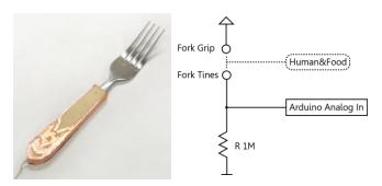
Figure 3: The prototype and circuit schematic of Digital EaTheremin.
