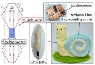
Figure 3. The prototype of the SmileSnail; The system swing the head by controlling wire 1 and 3; hang the head down/up with wire 2 and 4.
