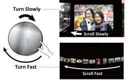
Figure 1. The concept of the IODisk. Users can control the speed/direction of digital contents in proportion to the rotating speed/direction of the disk.
