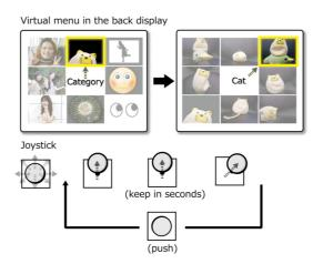
Fig. 8. Procedure for selecting content. Users can browse contents in the matrix menu by moving the joystick in 8 directions. They can select a content option by keeping the stick in the same direction for a few seconds. Information regarding the current category or content is shown in the back display.
