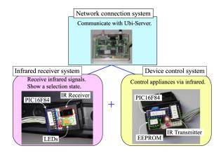
Fig. 5. System architecture of Attachable Controller.
