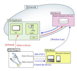
Fig. 2. System architecture of Ubi-Finger.
