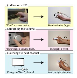
Fig. 6. Examples of operations using Ubi-Finger.
