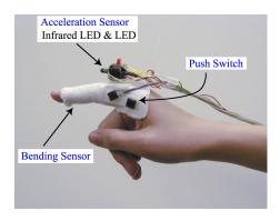
Fig. 3. Prototype of Ubi-Finger hardware.
